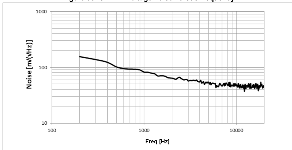
Figure 38. OPAMP voltage noise versus frequency
